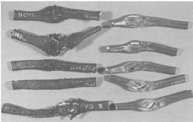
FIG. 1—Hammering of 14/2 copper cables.
